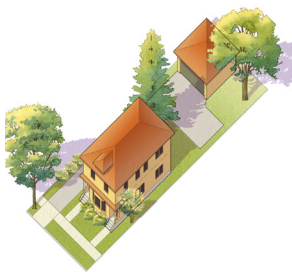
Figure 5.4 Duplex Stacked building type can create densities of 8-29 du/ac. For more explanation on density regulations, see Section 5.6.
